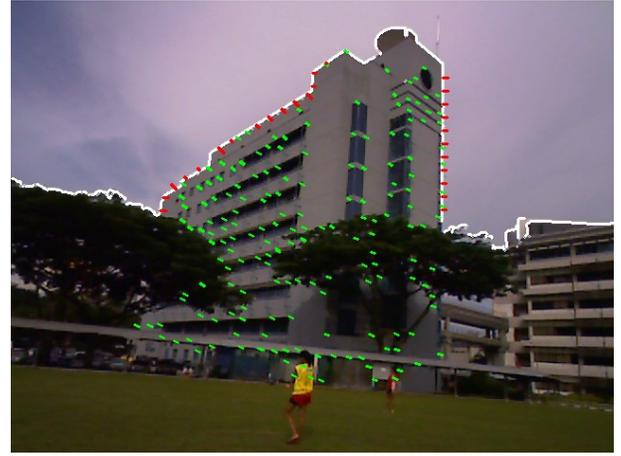
Figure 4: Combined feature tracking is in progress. Extracted silhouette from image is overlaid in white color. Edge correspondences obtained from model-to-frame tracking  $C_{MF}$  are illustrated with red color while green ones corresponds to frame-to-frame region based corner matching  $C_{FF}$ .
