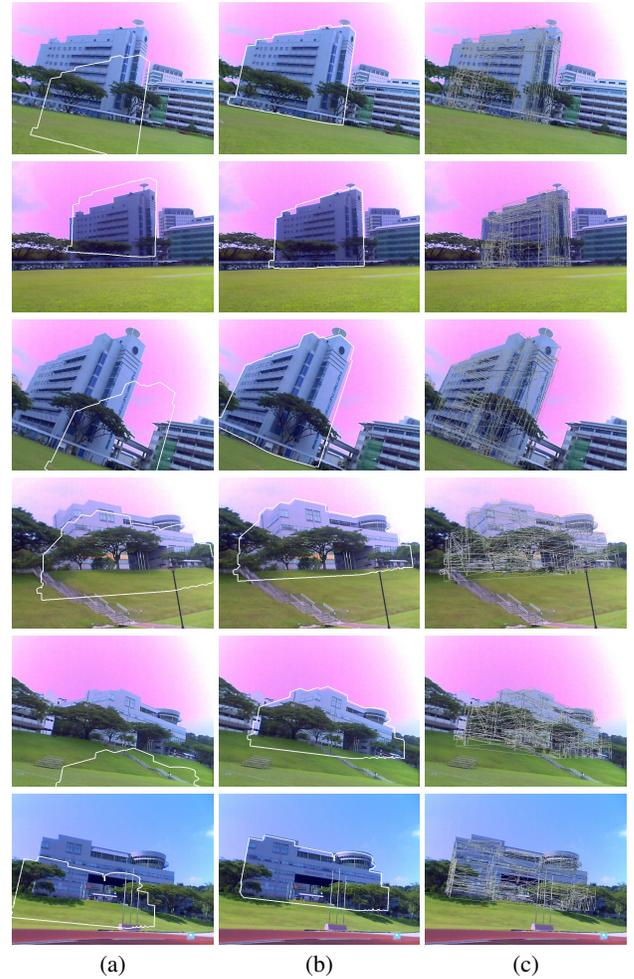
Figure 5: Results of one-step, model-based user positioning for different scenarios. The user is localized by shape context matching and WCLM optimization. (a) Coarse pose obtained from position and orientation sensors; (b) Corrected pose with superimposed silhouette; (d) Corrected pose with augmented wireframe of the model.
